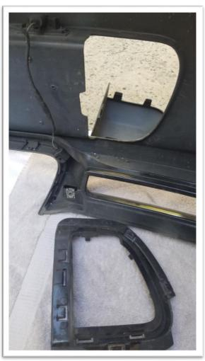
**STEP 3:** Clean thoroughly and apply 3M double sided tape to the top and bottom of the license plate holder. Next align and install license plate with the bumperette delete panel underneath.
