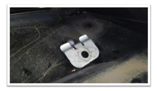
**STEP 4:** Raising the rear of the vehicle will assist in the removal of the final bolts but is not necessary. Locate the T30 bolt toward the top of the rear wheel well where the bumper and rear fender meet. Using the T30 screw driver or socket and extension remove this bolt and note the angle for reassembly. (**Fig.9**) Next, on the bottom side of the outer most edge of the bumper locate and remove the two T30 bolts. (**Fig.10**)
