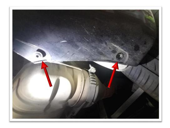
**STEP 5:** The final two T30 bolts are located on either side of the exhaust tip inside the bumper. **(Fig.11)**
