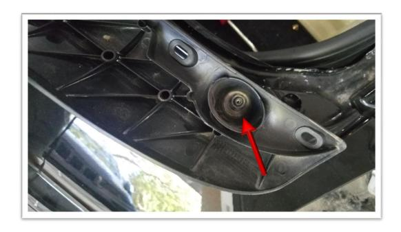
**STEP 3:** Locate and remove the two T30 bolts securing the bumper inside the tail light cavity. **(Fig.5)** The inner-most bolt will have a plate-washer under the bolt to be removed. Simply pull upward from the bottom and slide to the rear of the vehicle to remove. **(Fig.6,7,8)**
